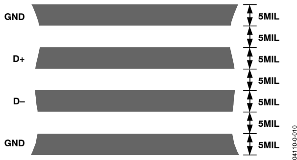
Figure 24. Typical Arrangement of Signal Tracks
